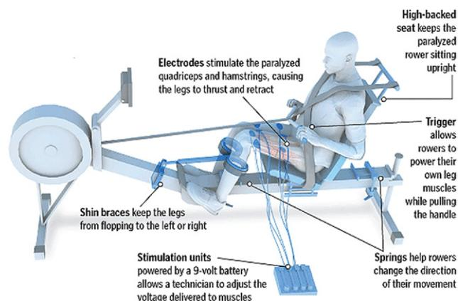
**Figure 1.** Schematic of adapted rower.
