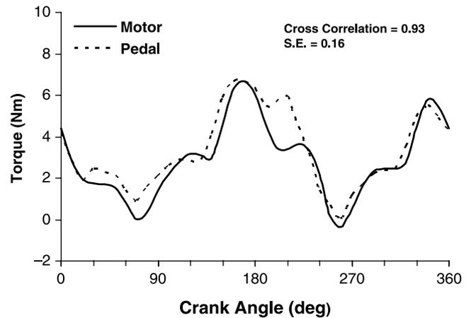
**Fig. 4.** Comparison of torque-angle curves from the instrumented pedals and the iFES-LCE for one subject. Cycle cadence was 20 rev/min. Torques generated from stimulation of R and L Quadriceps, Hamstrings, and Gluteal muscle groups. Cross-correlation function calculated at lag = 0 with standard error.
