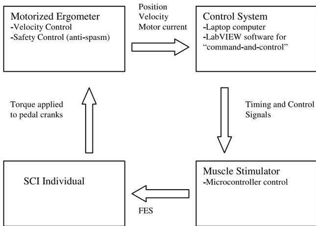
**Fig. 2.** Block diagram of components of the iFES-LCE with each component's basic function.
